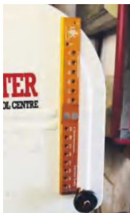
▲ This simple ruler scale makes it easy to set up veneer rips
